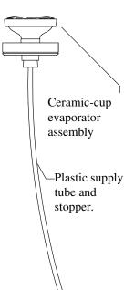
(3) Now clip the top assembly back onto the reservoir. Before snapping the top assembly down, fill the reservoir to the zero mark on the scale. (See a later page of these instructions for notes on Reading the Sight Tube.) If the
