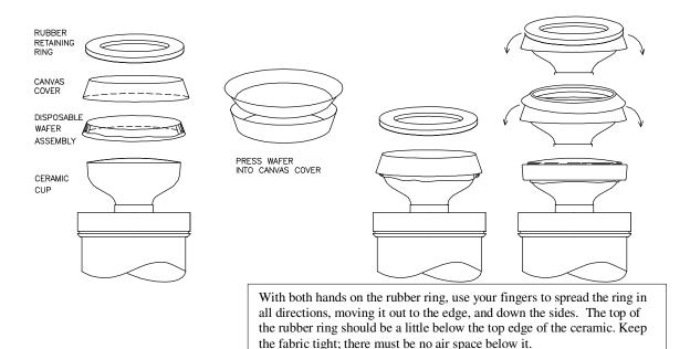
For low maintenance, use a disposable ETgage "wafer" between the green fabric cover and the ceramic evaporator surface. The wafer will protect the ceramic from accumulated contamination. When you remove a wafer, the ceramic should look wet.
