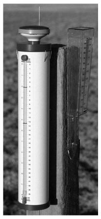
ETgage Model A, shown above, requires distilled water (available at food stores). Components of the system include: diffusion covers for grass ET (ETo) and crop ET (ETr), glass sight tube (inches and mm), stainless steel mounting bracket, rain gauge, bird-wires, instructions, irrigation management information and tables.
